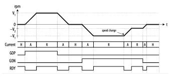
speed will ramp linearly to the target speed. The GOP input has priority over GON input.
